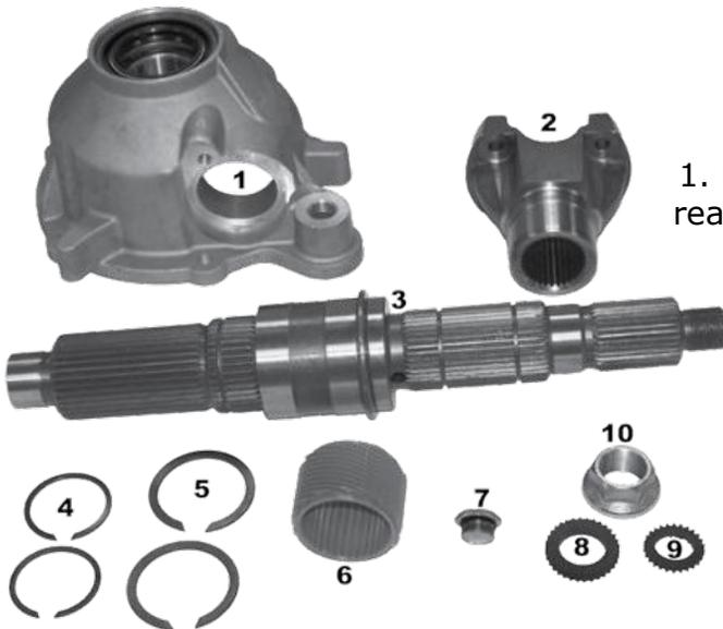
1. Rear Housing Assembly (Includes rear housing, rear output seal, rear output bearing and rear output snap ring, pre-assembled.)
