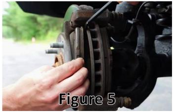
Remove the caliper bracket from the knuckle using a 21mm socket or wrench. See Figure 6.
